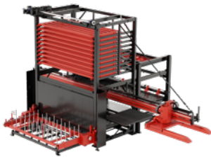
ASR-PR Single tower L/UL + part removal
