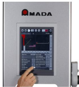
The NC control is capable of generating programs automatically. It takes into account bending constraints and ergonomics, including gauging position, component handling, bend order and required tolerance
