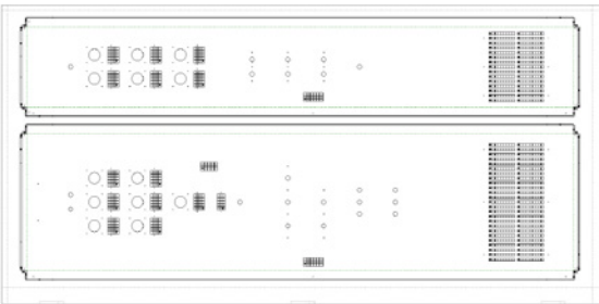
Galvanised steel 2.3 mm 2438 x 1219 mm
